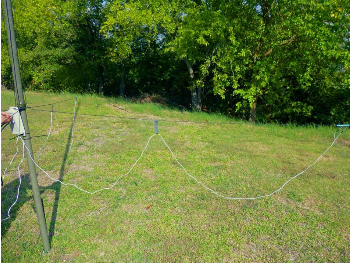
Coupler transmission line is kept clear of ground and other loop transmission lines
